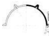
Sectional drawing of segment. PA/PE 5 and PA/PE 6 Ring with a total of 6 skids
